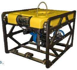
The Sea Rover's onboard systems communicate through a 10GB ethernet backbone with a fiber optic connection to the surface station. Sea Rover's open Unistrut and Delrin frame is a simple, secure frame for multiple accessories.
